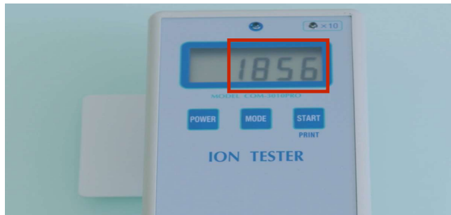
Number of ions measured by the negative ion measuring instrument “COM-3010PRO” 1,856/cm 3
